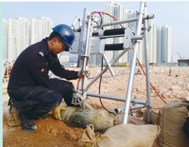
爆炸品處理課人員利用水力磨沙切割系統處理一枚美軍 100 磅空投炸彈。 An Explosive Ordnance Disposal officer renders a 100-pound aircraft bomb safe with the assistance of the Abrasive Water Cutting System.
