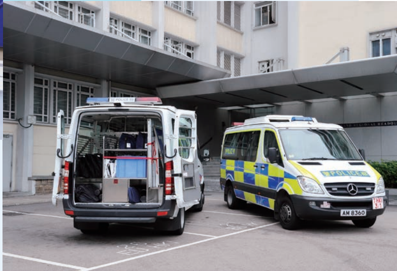
全新大型客運貨車的尾部均劃一配置裝備架。 All new large vans are fitted with a load-carrying system at the rear.
