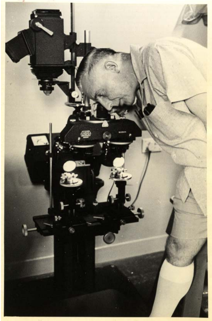
Leitz Comparison Microscope for comparing fired bullets, which is now displayed in the Police Museum
